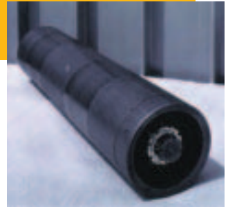
Graphite sleeve surrounding "natural uranium" GCR fuel
