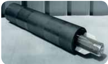
A graphite sleeve surrounding the fuel used in first generation nuclear reactors
