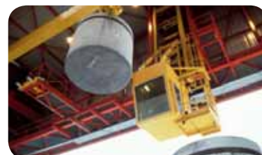
Disposal of an LILW-SL package in a cell at the waste disposal facility for short-lived, low- or intermediate-level waste (CSFMA)
