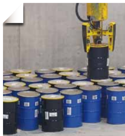
LILW-SL package disposal at the Aube facility
