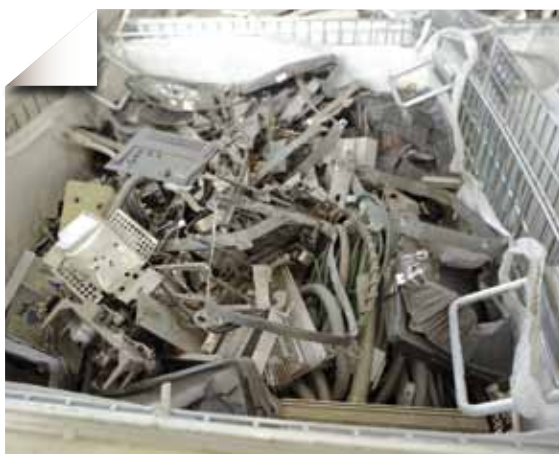
Industrial VLLW (such as scrap metal and plastics) before conditioning
