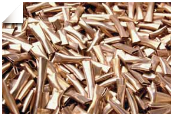
Metallic waste from the structures surrounding spent fuel (hulls and end caps).
