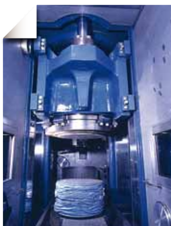
Compacting a drum of LILW-SL
