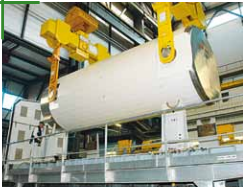
TN28 casks used to transport CSD-V packages to Belgium, the Netherlands and Japan
