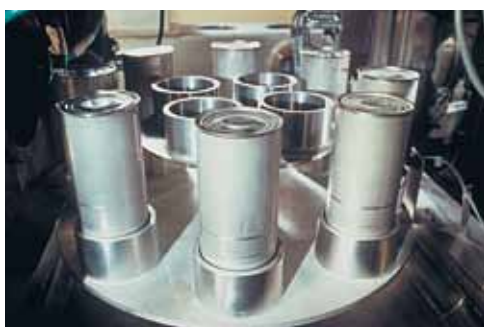
Carousel of plutonium cans at the AREVA Melox MOX fuel manufacturing plant at Marcoule
