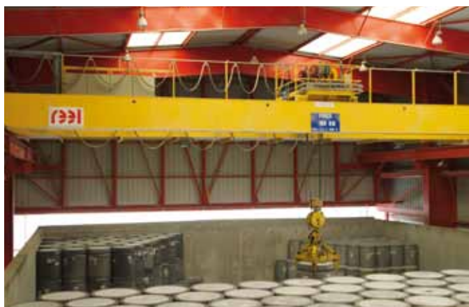
Lowering a concrete package into a cell (LILW-SL disposal facility)
