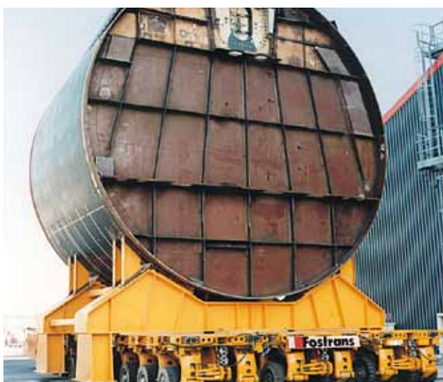
Submarine Le Redoutable: cross section of the submarine's reactor unit
