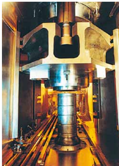
Hull compacting unit (ACC) in the AREVA plant at La Hague (Manche district)
