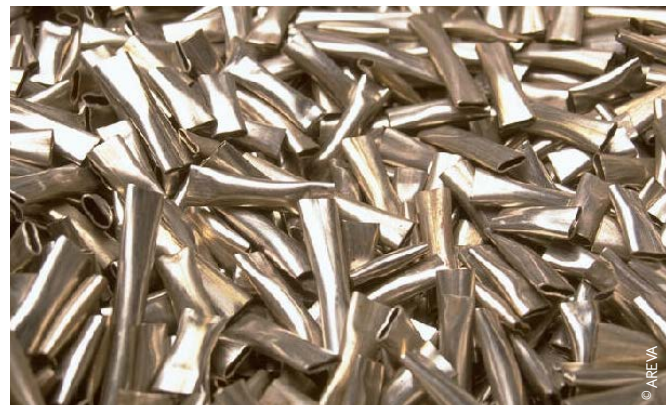
▲ Metallic waste from the structures surrounding spent fuel (hulls)
