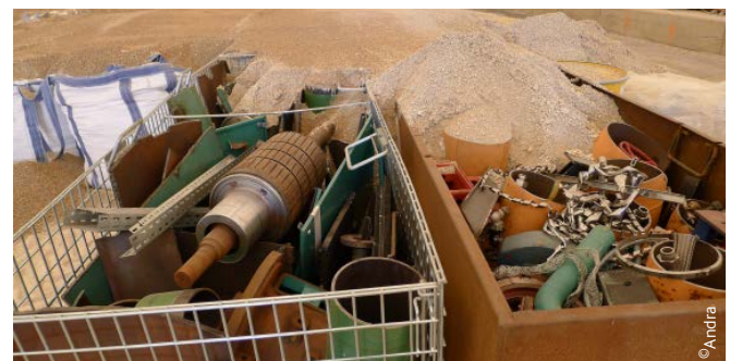
Disposal of VLLW metallic waste in a cell at Cires
