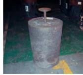
Melting metal waste SOCODEI/CENTRACO <sup>Cast ingot</sup> 128/129
