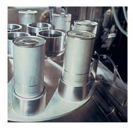
Carrousel of plutonium cans at AREVA's MOX fuel manufacturing plantat Marcoule
