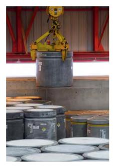
**Concrete packages of cemented waste**
