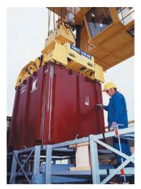
Metal container box filled with cemented waste
