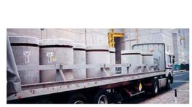
**Concrete packages of cemented waste**
