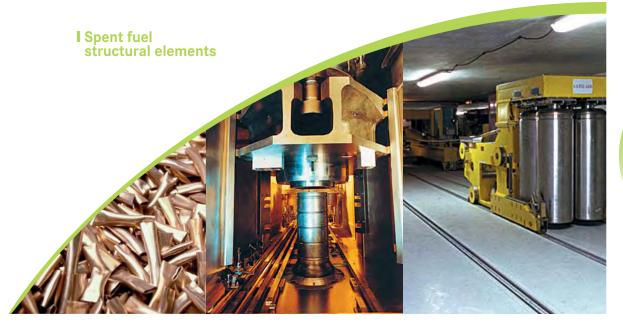
The first step in spent fuel processing consists in shearing and dissolving the material contained in the structural elements. Once emptied, these elements are still radioactive and are considered as waste. They are sometimes called "hulls and end caps". This type of waste was cemented in the past but is now compacted at AREVA's La Hague hull compacting facility. They are then placed in stainless steel containers (called "CSD-Cs") and stored at the La Hague site.
